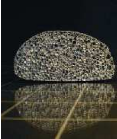
Figure 6. An example of foamed zinc. The bubbly melt must be solidified quickly to retain the homogeneous structure, a structure not required in the microgravity environment. Image courtesy of J. Banhart.
