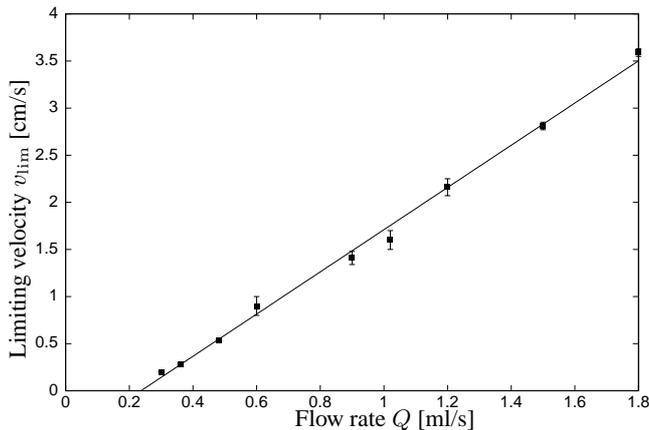
**Fig. 4.** The limit velocity  $v_{lim}$  reached by the convective roll in a tilted tube varies linearly with flow rate. Extracted from the data of figure 3.
