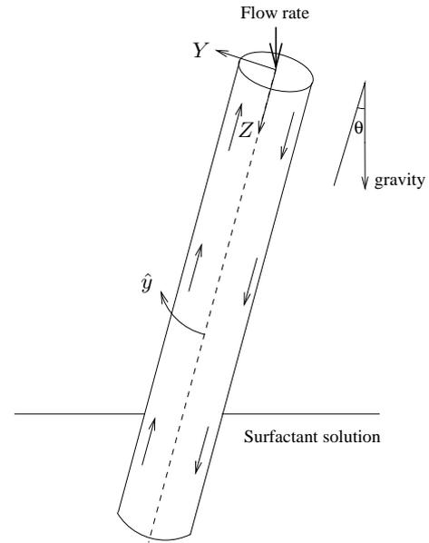
**Fig. 1.** A sketch of the convective roll in a tilted tube, showing the  $(Y, Z)$  coordinate system used in the analysis and the  $\hat{y}$  coordinate around the cylinder. The dashed central line is a reference showing the central axis of the tube. The arrows show the sense of the motion of the bubbles. Fluid draining into and through the foam moves preferably in the vertical direction, due to gravity.
