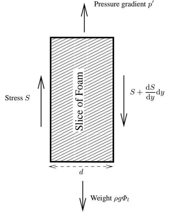
**Fig. 6.** The forces acting on a small element of the foam. The weight of the foam,  $\rho g \Phi_l$ , is balanced by the pressure gradient  $p'$  and the shear stresses on the wall.
