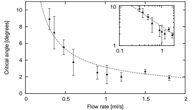
**Fig. 5.** The motion of bubbles in the tilted tube begins, for given flow rate  $Q$ , when the angle of tilt is increased beyond a critical value  $\theta_c$ . The solid line is a fit to the form given in (17),  $\theta_c \propto Q^{-3/4}$ , with a coefficient of proportionality of  $3.17 \pm 0.17$ . The inset shows the data on log scales.
