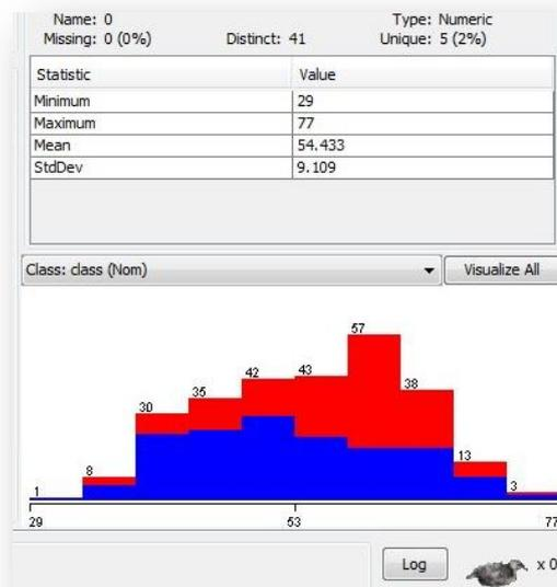
If the feature is discrete, then a bar chart of the frequencies of its values is displayed. If it's continuous (as in the figure above), then the distribution of values will be displayed. The 'Visualise All' button shows the visualisation for all features in the dataset.
