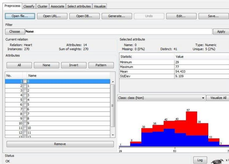
Once the dataset has been loaded, you are presented with a range of information. This window is the 'Preprocess' tab, where the dataset can be processed, e.g. feature selection applied, instances removed, missing values removed etc. On the bottom-left of the screen there is a list of features in the dataset:
