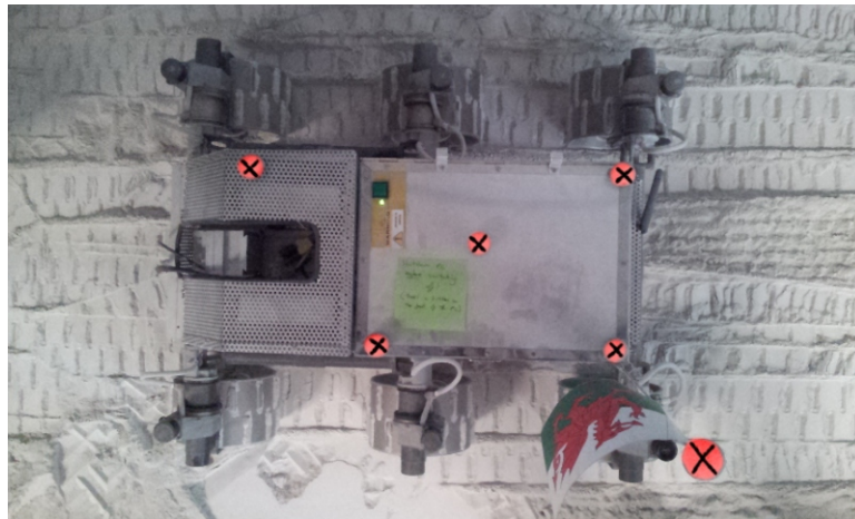
Figure 2.4: The positions of the fiducial markers on the rover, shown in red with crosses.
