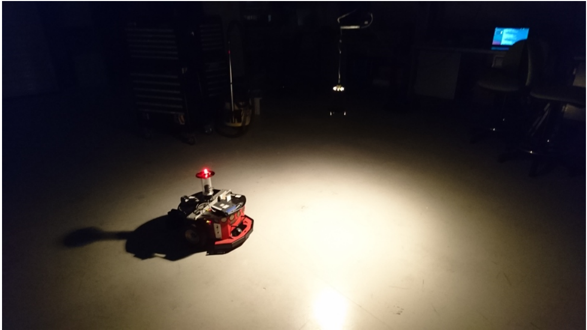
Figure 10.2: The robot and its light source during an experimental run. The red LED is used for tracking.
