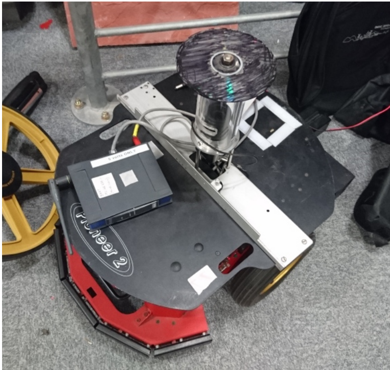
Figure 8.1: “Bart”, the Pioneer 2-DX robot used in the experiments. Note the camera, which is pointing upwards into a parabolic mirror mounted in an acrylic tube.
