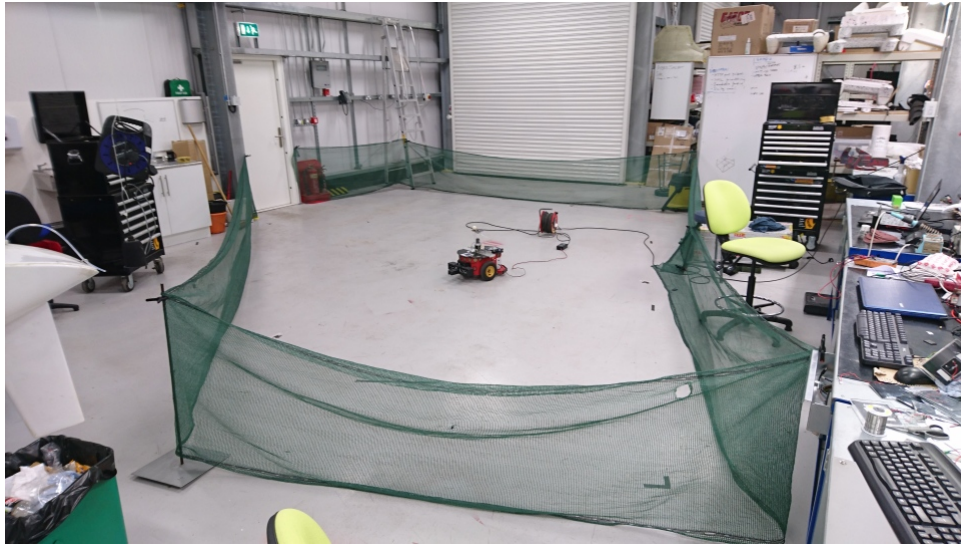
Figure 8.2: The robot inside the experimental arena, which is bounded with sonar-opaque mesh. The mesh in the left of the image was positioned slightly differently in the experiments as shown in Fig. 10.1, and was held taut by clips during the runs.
