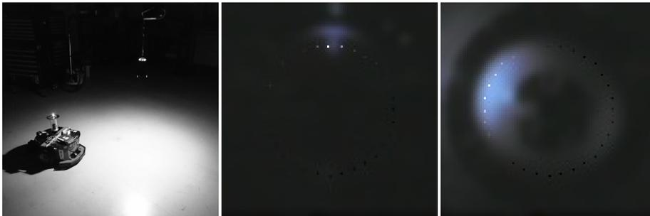
(a) Robot and light source      (b) Camera image, blurred, far light      (c) Camera image, blurred, near light
