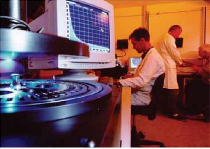
Fig 6 (left) Typical OSL signal observed from a quartz aliquot – the OSL signal drops rapidly as the trapped electrons in the quartz are used up to produce the luminescence signal. (right) An automated luminescence reader equipped with blue-light-emitting diodes (LEDs). When in use, the lid closes, leaving the sample holder in darkness. The blue LEDs are switched on to measure the optically stimulated luminescence (OSL) signal (© Risø National Laboratory, Denmark).
