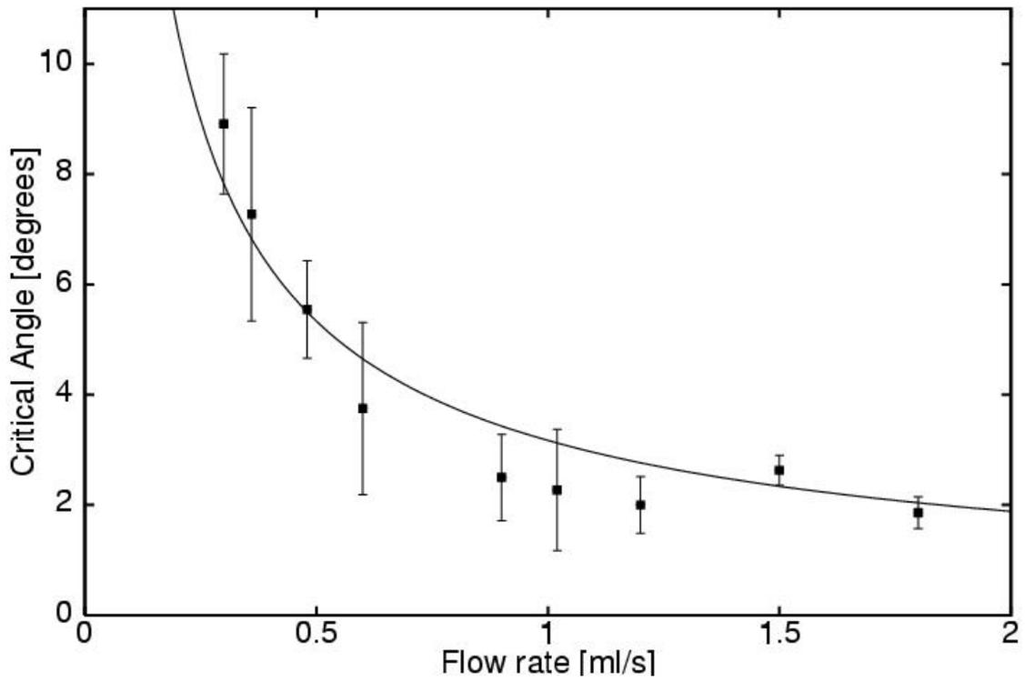
**Figure 4:** The motion of bubbles in the tilted tube begins, for given flow rate  $Q$ , when the angle of tilt is increased beyond a critical angle  $\theta_c$ . The solid line is a least-squares fit to the theoretical prediction of eqn. (1).
