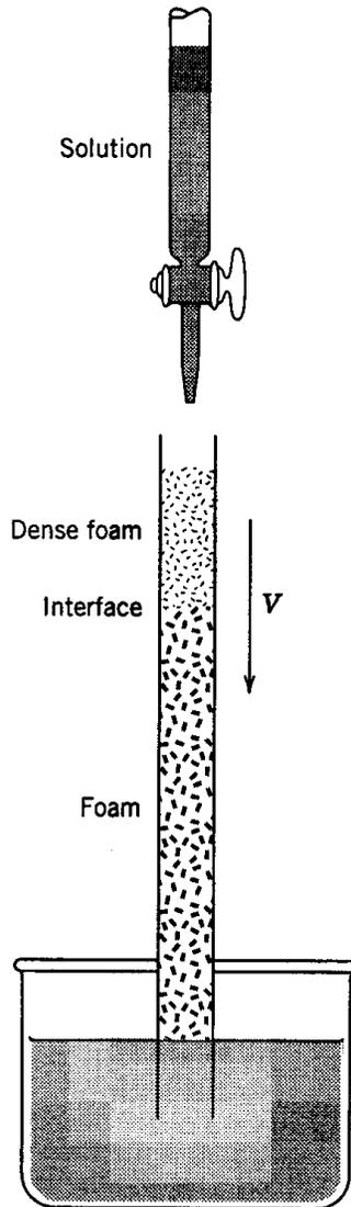
**Figure 1:** In forced drainage experiments surfactant solution is added to a dry foam at a fixed flow rate. This results in the propagation of a drainage wave through the foam, leaving in its wake a column of foam with a constant liquid fraction. For high enough flow rates convective bubble motion is observed.
