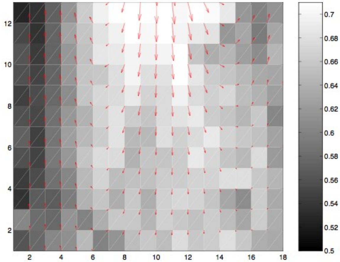
**Figure 6:** Velocity field (arrows) and density profile (grey levels, in arbitrary units, indicative of the wetness of the foam) obtained for the Hele-Shaw set-up of figure 5 and a point input of surfactant solution. Data was taken once a steady liquid density profile was established. The data is averaged over 20 seconds (spatial average roughly two bubble diameters).
