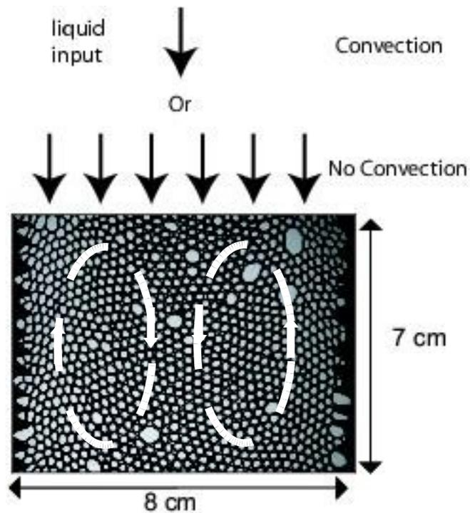
**Figure 5:** Set-up for the study of convection in a Hele-Shaw cell filled with a monolayer of bubbles (spacing of glass plates: 1.5mm, mean distance between centres of neighbouring bubbles:  $2.4 \pm 0.2$ mm). The bottom of the cell (not shown) is submerged in a pool of surfactant solution, the total height of the cell is 20cm. For a uniform input of solution no convection is observed. Input at the midpoint of the upper edge of the cell leads to two counter rotating rolls, as sketched.
