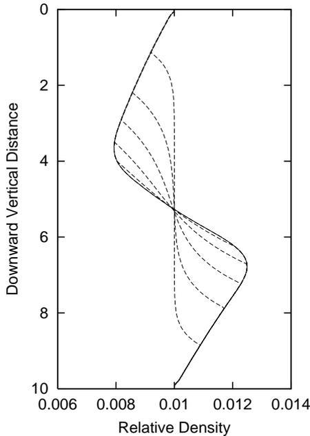
**Fig. 3.** Successive profiles of relative density are shown for case I, starting from a liquid foam with constant liquid fraction  $\Phi_1^0 = 0.01$  and  $Pe = 1$ . Dashed lines denote the profiles at time intervals of  $\tau = 20$  and the solid line is the eventual, frozen, profile at  $\tau = 140$ .
