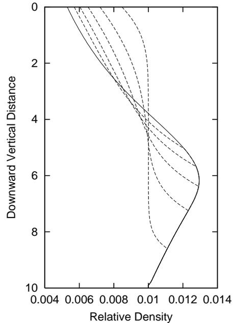
**Fig. 4.** Successive profiles of relative density are shown for case II, starting from a liquid foam with constant liquid fraction  $\Phi_1^0 = 0.01$  and  $Pe = 1$ . Dashed lines denote the profiles at time intervals of  $\tau = 36$  and the solid line is the eventual frozen profile at  $\tau = 450$ .
