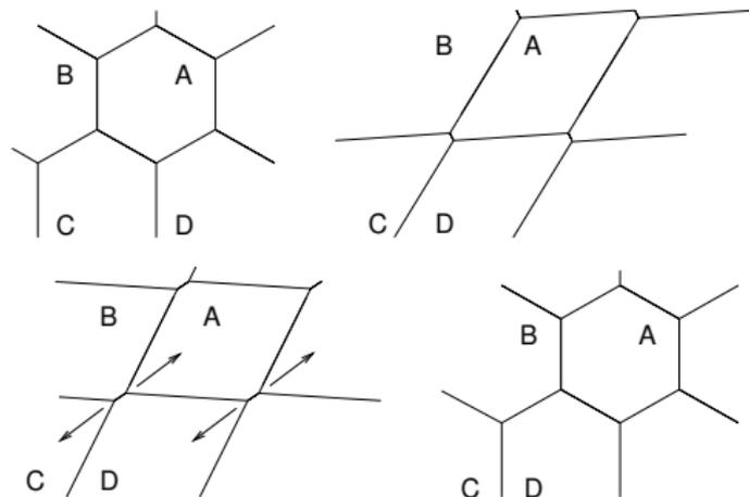
Under shear, system undergoes *topological transformation*
