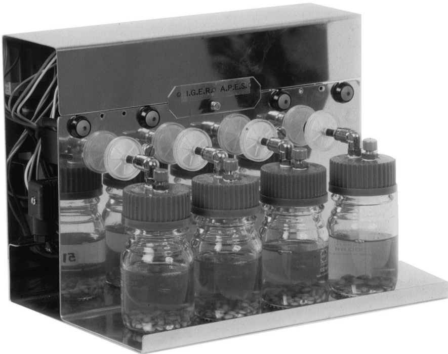
Fig. 1. One rack of four bottles of the automated pressure evaluation system (APES).
