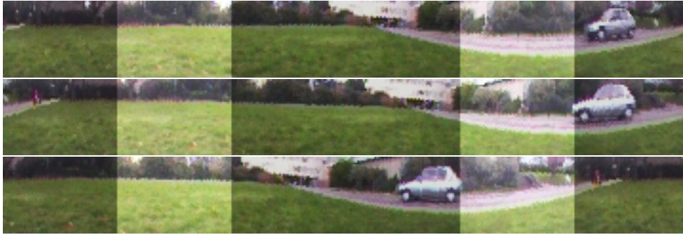
Figure 22: GRASS2: the panoramic images corresponding to frame 51 (top) and frames 52 and 53 (middle and bottom) after un-rotation using the global minimum of the distance function in Figure 21. The light bands correspond to the kept field of view.
