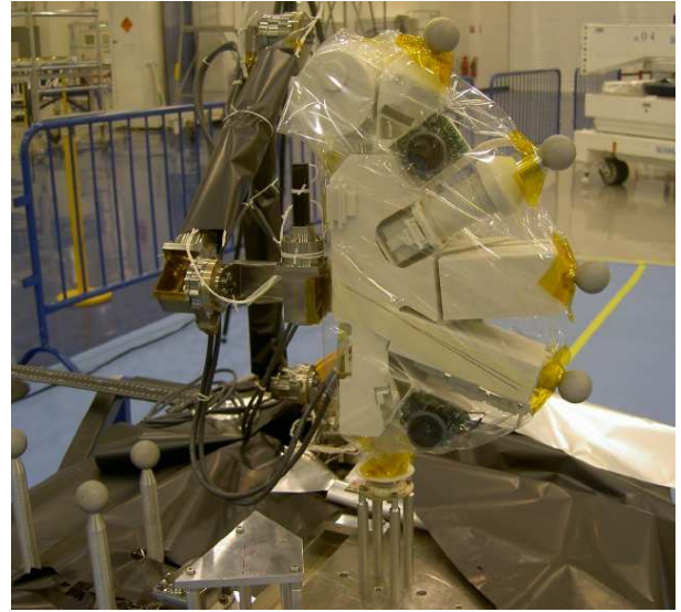
Figure 13: FM ARM and 1/3rd mass PAW shown after being commanded to position the mole in the GAP inlet port using Envision(TR) generated ARM joint data.
