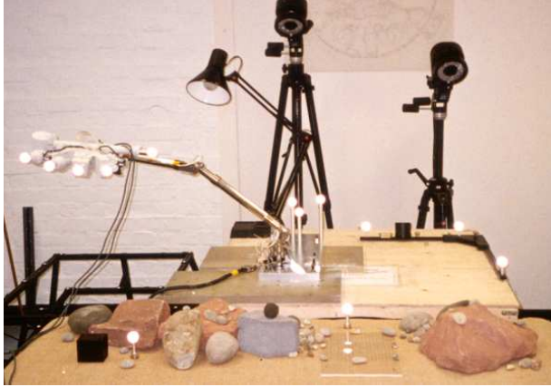
Figure 3: Calibration setup with the Beagle2 DM ARM, 1/3rd mass PAW, and mock terrain.
