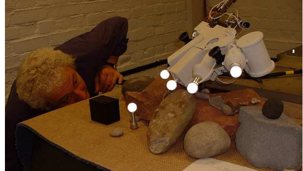
Figure 11: End-to-end DM ARM and 1/3rd mass PAW tests using virtual ARM/PAW model, and mock terrain.
