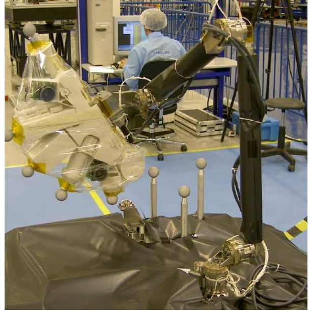
Figure 4: Calibration setup with the Beagle2 FM ARM and 1/3rd mass PAW in Astrium Ltd. clean room.
