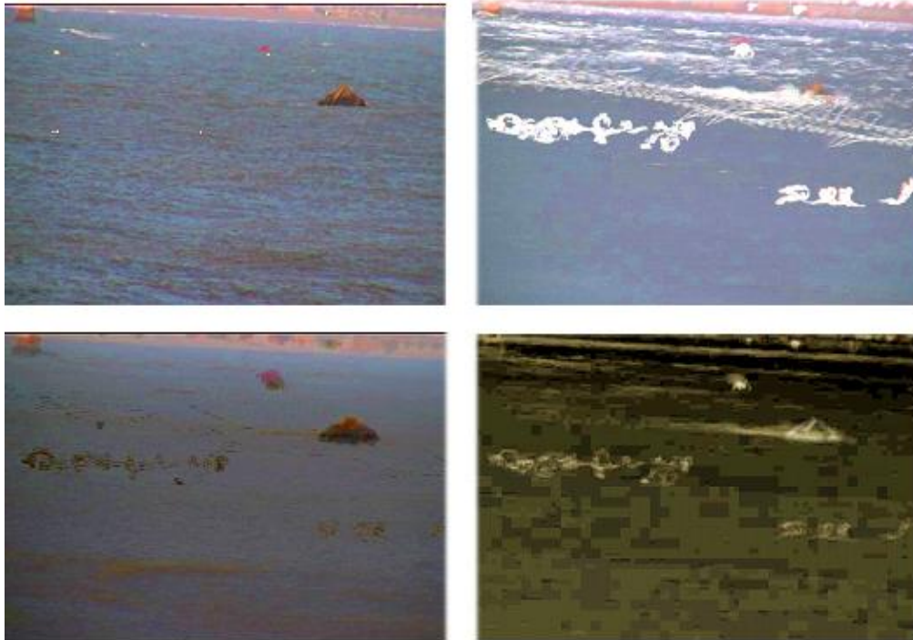
Figure 4. Temporal processing on sea images. (Top Left) One of the original images. (Top Right) Maximum DN at a given pixel – the wiggly lines are sea gull take offs and landings. (Bottom left) Minimum DN. (Bottom Right) Standard deviation DN. From Vickers (2006).
