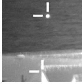
Figure 5. Section of image used to measure the wave height of the buoy. The lower and upper markers define the origin and the buoy.
